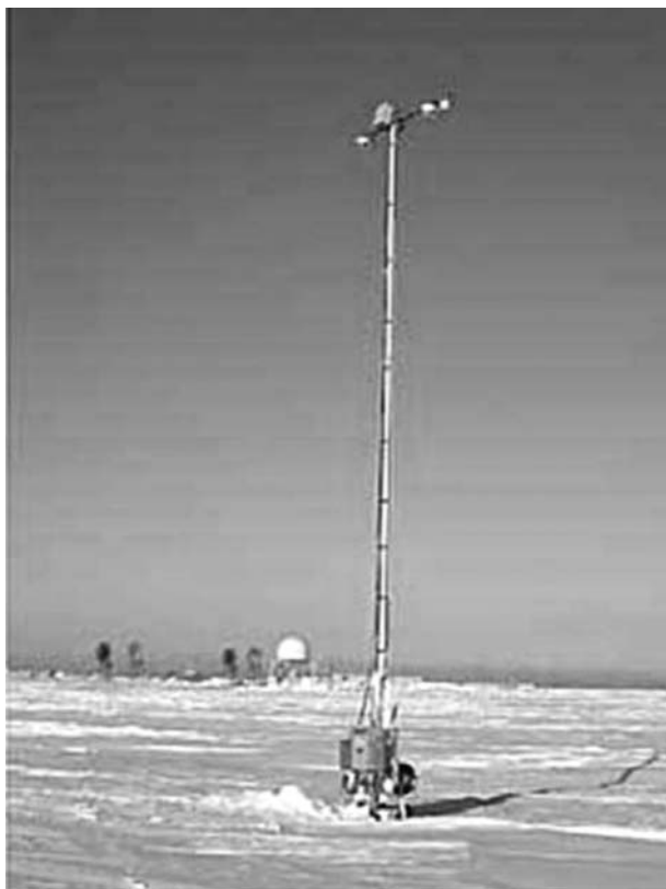
Fig. 1. Photograph of the upward and downward viewing radiometers used to determining the snow albedo at the North Slope Barrow, Alaska (USA), ARM site. Source: http://www.arm.gov/instruments/instrument.php?id=15
